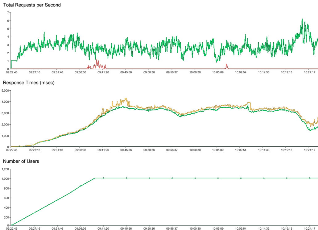
Figure 2: Total requests per second (green) and failures per second (red) – top figure; maximum response time (ms) in the particular second (yellow) and the median response time (ms) (green) – middle figure; number of users that are active (total 1000 users) – bottom figure
